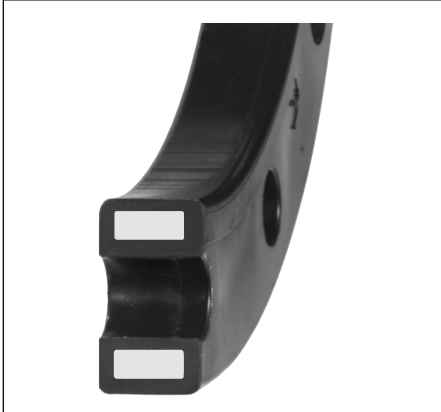
Sectional sketch showing the wallthickness of the coating and the metal core (no diffusion).
