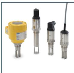
Principle: Contact to liquids dampens the vibrating fork which activates the alarm contact
