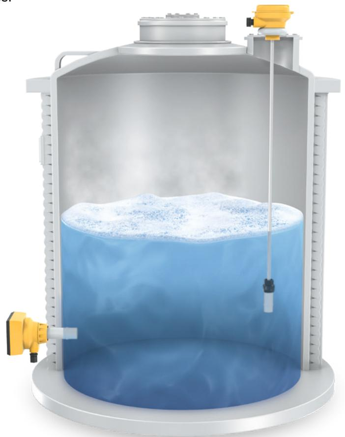
Mounted through the tank wall or submersed from the top of the tank, a hydrostatic sensor measures the weight of a fluid column. The change and therefore the pressure at the sensor is proportional to the change in the tank level. A capillary tube in the cable ensures that changes of the atmospheric pressure can be compensated.
