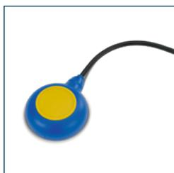
The type 2285 floats on top of the fluid being measured due to its relative density being less than that of water. The level switch is triggered when the internal contact reaches the +/- 45 from horizontal switching angle.
